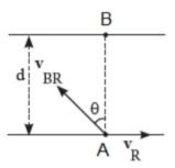
$V_{\text{BR}}$  is velocity of boat wrt water or velocity of man wrt water,  $V_{\,\text{R}}$  is velocity of river.
